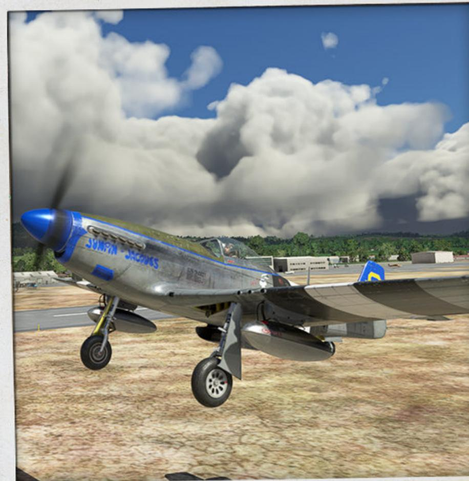
Once the plane is in the air the P-51D becomes a totally different and graceful machine. Unlike the spitfire Do not apply brakes to stop the wheels from rotating. Take this time to ensure that the manifold pressure is set to around 46 inch mp and RPM back to around 2700 rpm . The plane will climb at the speed of 160 - 170 mph fine.
